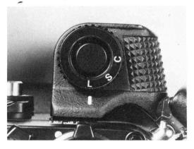
achieved by switching both the motor drive and camera on and using the camera's shutter-release button rather than the MD-4 shutter-release. The speeds at which the MD-4 will operate, varies depending on the power source and whether or not the mirror is locked up. Top speeds are reached with NiCd batteries (5.5 fps normally and 6 fps with the mirror locked up). With AA alkaline batteries top speed is 3.8 fps and 4 fps with the mirror up.
