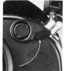
To make multiple exposures, make the first exposure normally, then before advancing to the next frame, push the multiple exposure lever counter-clockwise. Turn the advance lever and the shutter will be cocked but the film will not advance.
