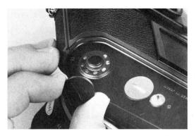
To mount the MD-4 motor drive, you must first remove the rewind cap on the camera's baseplate.
